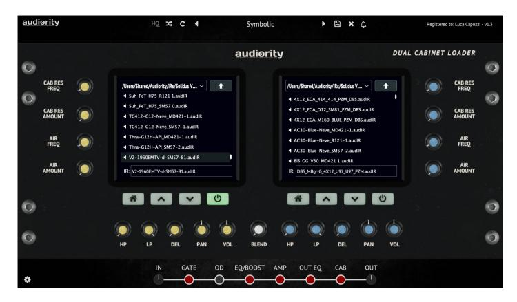
A dual cabinet simulator / IR loader. It can load our custom ".audIR" files or standard WAV files.
