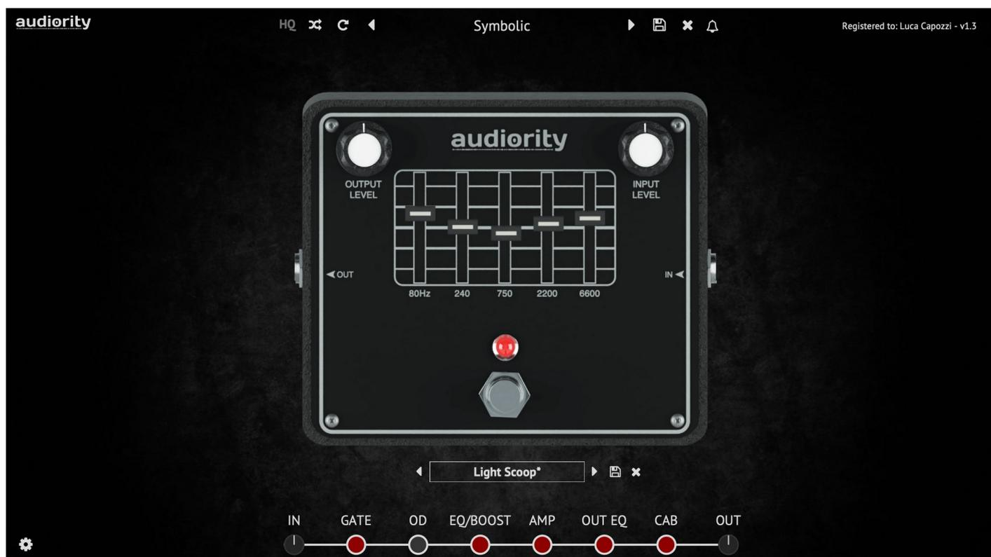
A post-amp five band equalizer to shape the amp sound before going to the cabinet.
