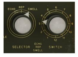
The **SELECTOR** and **SWITCH** knobs form the switching circuitry. The **SELECTOR** knob allows selection between **ECHO**, **REPEAT** and **SWELL**. **ECHO** is just one repeat; **REPEAT** is multiple repetitions, depending on the "**LENGTH OF SWELL**" knob; **SWELL** is pretty much like **REPEAT**, but introduces a little signal from all four playback heads in the mix. That's very useful to reproduce reverb type effects.
